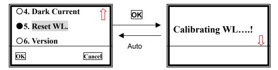
Fig. 2-8 Calibrate Wavelength
