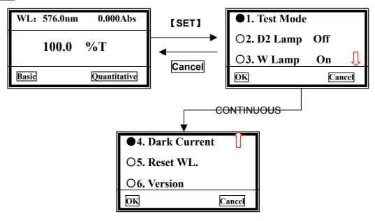
Fig.2-3 go into utility setting interface
